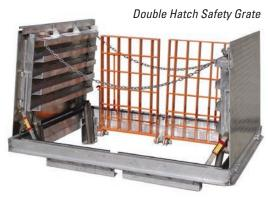
For large openings, USF Fabrication makes a dual safety grate that hinges on opposite sides of the hatch frame and double safety grate that hinges on same side of the hatch frame. These configurations can place a barrier on three sides of the hatch's opening. A safety chain can be employed to block the fourth side of the opening.
